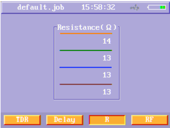
Figure24 Auto test d. c. loop resistance results menu
