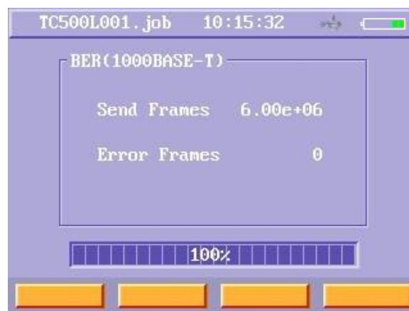
Figure37 Data cable BER test menu
