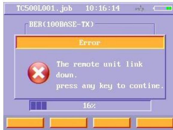
Figure38 Data cable BER test menu (error)
