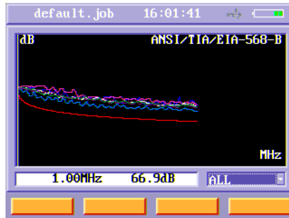
Figure36 Data cable NEXT manual test result menu
